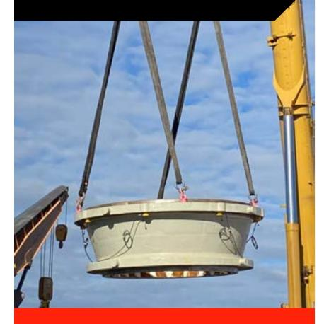
The Rotable shell solution is available for any Superior<sup>™</sup> gyratory crusher.
