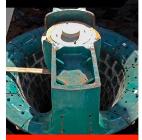
The Super spider has been developed for 4265, 5475, and 6089 size Superior™ gyratory crushers.
