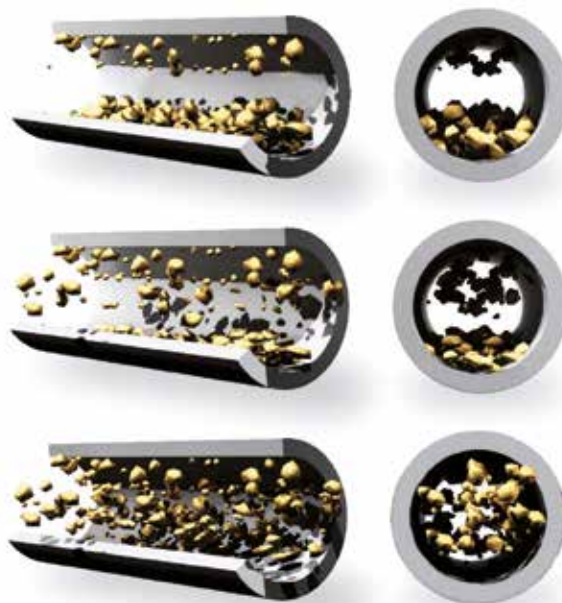
Figure 3: Different flow conditions. The lowest variant represents the preferred flow conditions.
