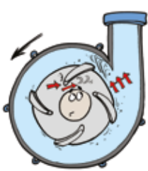
Below BEP operation
