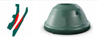
Example of normal wear. Obtained with correct feed arrangements, feed gradation and parameters for the cavity.
