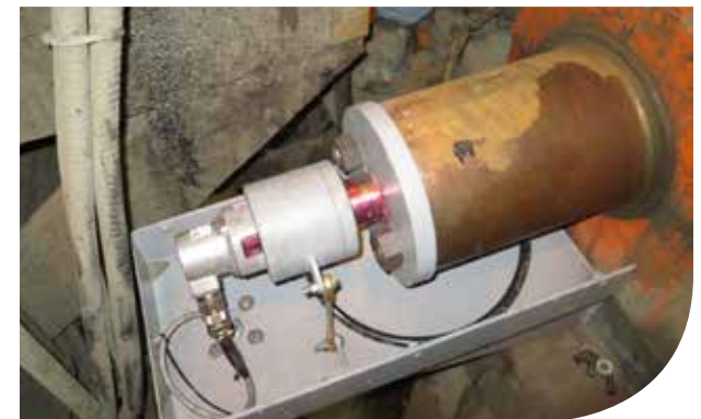
Exposed pinion shaft encoder
