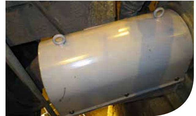
Housing for pinion shaft encoder
